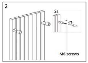
Figure 3 | Fixing the radiator brackets
