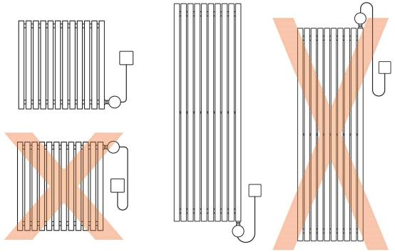
Figure 1 | Correct and incorrect element positioning
