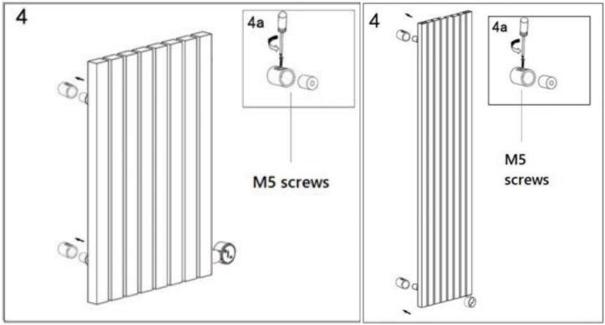
Figure 5 | Securing the radiator to the wall (horizontal and vertical)
