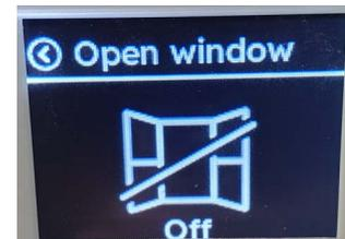
In this setting you can deactivate open window detection or activate it and set how long the radiator waits before switching back to the full set temperature. Open window detection is disabled by default.
