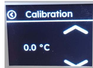
The accuracy of the radiator's temperature reading can be affected if the unit is mounted with the sensor in a hot or cold spot, such as hot water pipes or a draughty doorway. The sensor is at the bottom of the unit.
